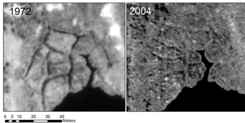
Figure 8 An example of a high-centred polygon field (69.444°N, 132.951°W) showing a decrease in melt pond area from 1972 to 2004.
